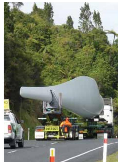
*A 53m blade being driven along SH23 to Raglan for the Te Uku Wind Farm (2010)*
